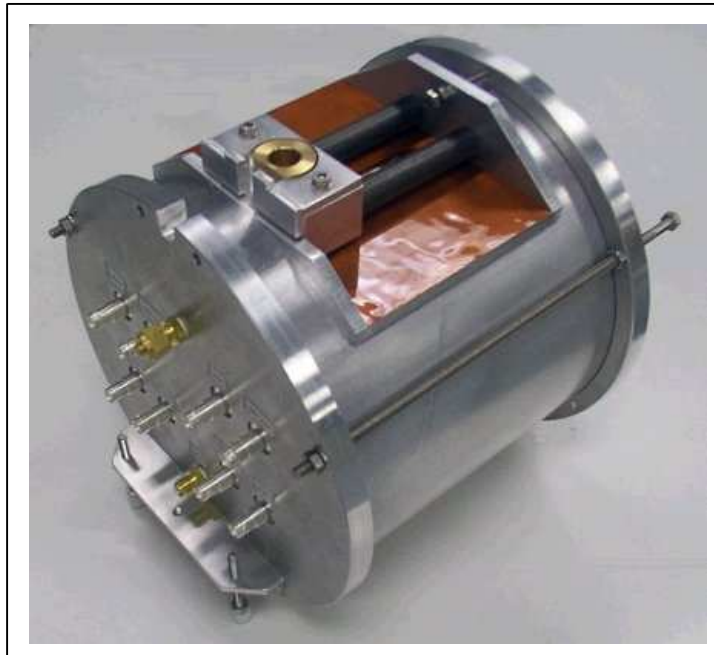
Fig.3 The new GEM based Mini-TPC for current measurements in the 5 Tesla magnet
